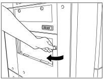
Put down the lower guide of the exit side and remove any misfed paper.
